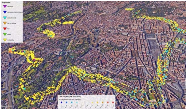
Rome Walls deformation satellite monitoring © Spizzichino
