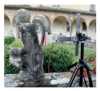
Fig. 2 Microwave heating treatment of biodeteriogens growing on stone
