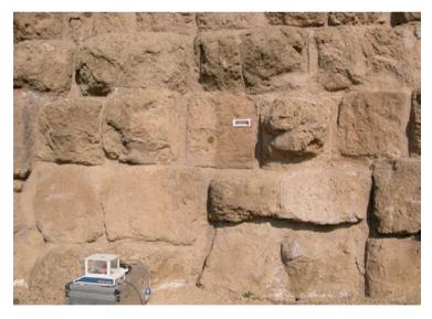
Fig. 4 Contact sponge test: on site analysis for investigating the amount of water in different areas and the change of water surface distribution after the application of consolidating products on Servian Wall in Rome
