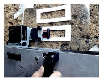
Fig. 1 Peeling Test Device system aiming to measure the removed material using a tape, and the necessary strength to remove it
