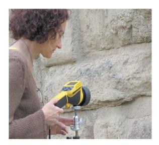
Fig. 2 Infrared thermography applied on the Servian Wall in Rome
