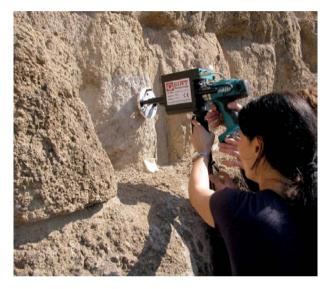
Fig. 5 Drilling resistance measured by DRMS: on site analysis on areas with different consolidation treatments on the Servian Wall in Rome
