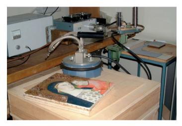
Fig. 1 Microwave heating treatment of woodworm disinfestation
